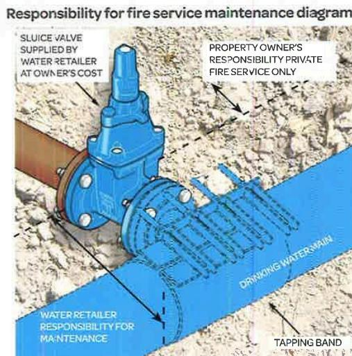
**Note:** The property owner is responsible for the connecting bolts/nuts/gasket and piping into the property from the outlet of the sluice valve
