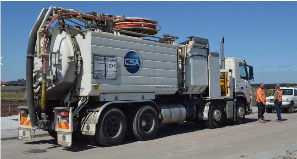
Figure 9 - Combination truck - driver side
