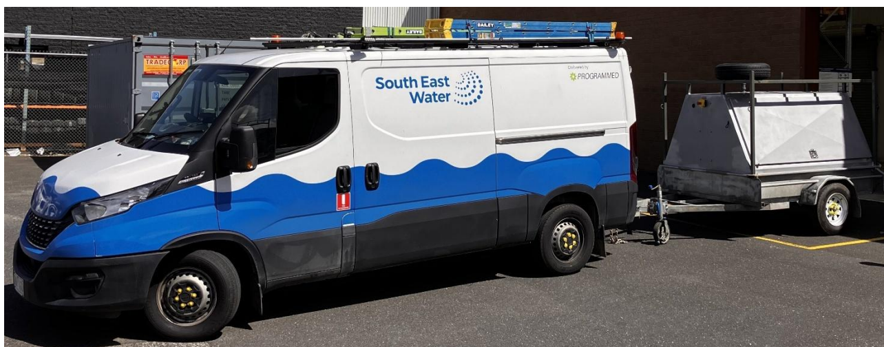
Figure 14 - Hypo delivery trailer towed by a van
