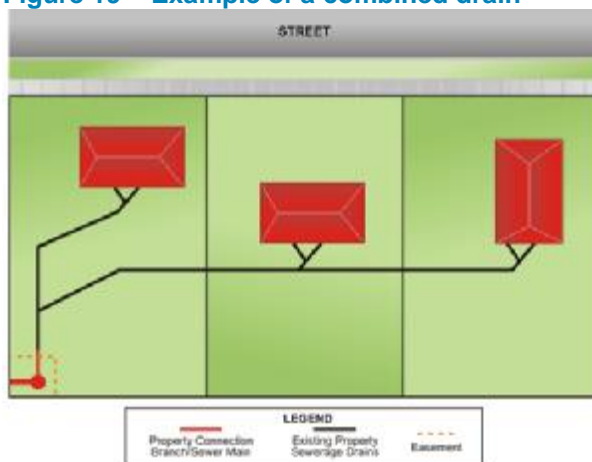
Figure 20 – Two residences relieving a combined drain
