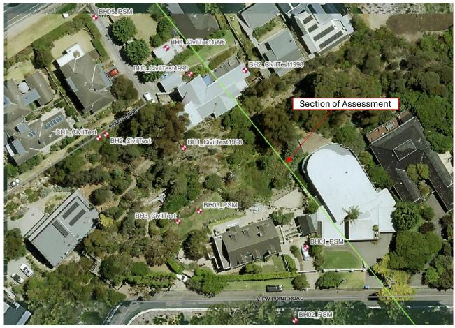
Figure 6: Layout of assessed boreholes
