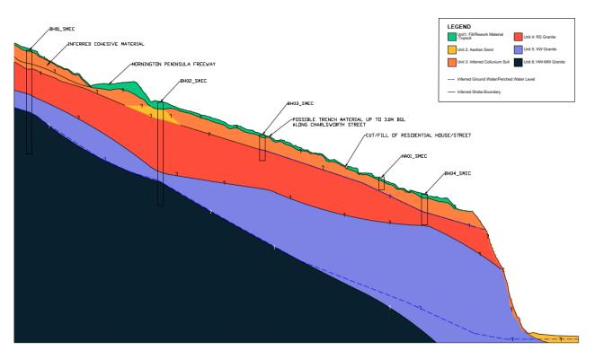
Figure 30: Cross-sectional sketch of the vicinity of the McCrae Landslide showing distribution of geotechnical units (not to scale).
