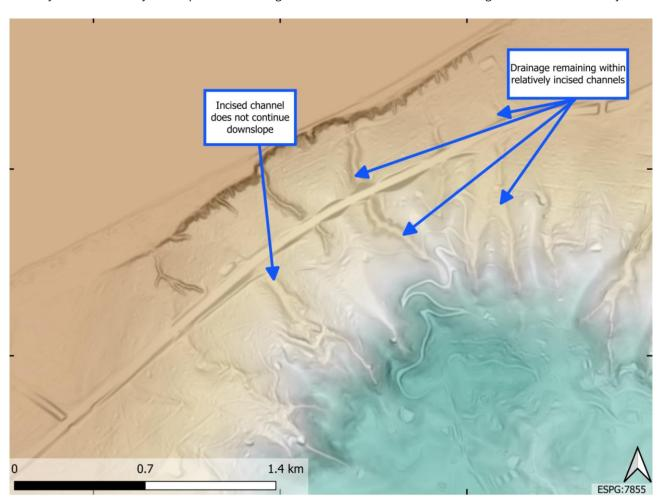
Figure 33: Plan showing DEM modelling and LiDAR survey information in the McCrae region (DEM source: Geoscience Australia, DEM of Australia derived from LiDAR 5 Metre Grid)
