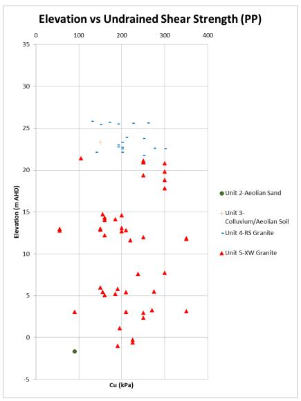
Figure 14: Pocket penetrometer result plot
