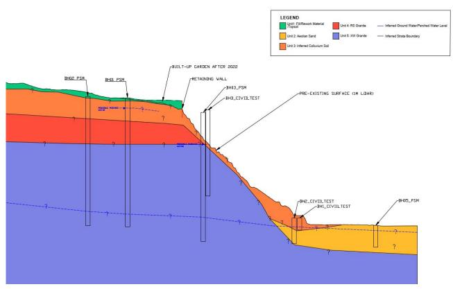
Figure 29: Cross-sectional sketch of the escarpment at the McCrae Landslide showing distribution of geotechnical units (not to scale). Note PSM BH03 is offset approximately 25m to west of cross-section.
