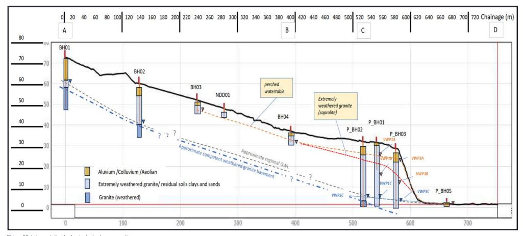
Figure 32: Interpretative hydrogeological cross section
