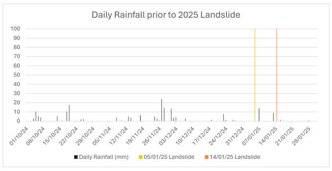
Figure 7: Daily rainfall prior to 2025 McCrae Landslide at 10-12 View Point Road
