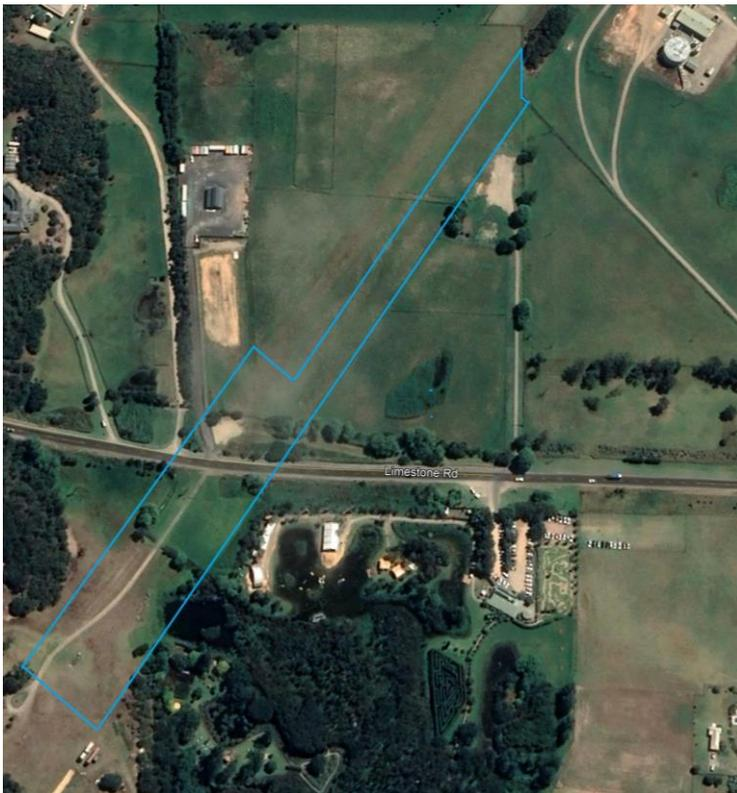
We have been assessing different options for this planned connection with in principle agreement on the design being reached with Melbourne Water in early February 2019. While we had proposed to connect into the SEO pipeline as it runs adjacent to our plant, Melbourne Water has advised us that we need to connect into the existing manhole at 725 Limestone Road with the pipeline located within the existing SEO easement (see map below).
