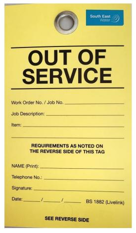
Figure 8: Example Out of Service Tag
