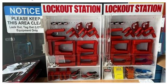
Figure 14: Extra-Large Enclosed Lockout Stations
